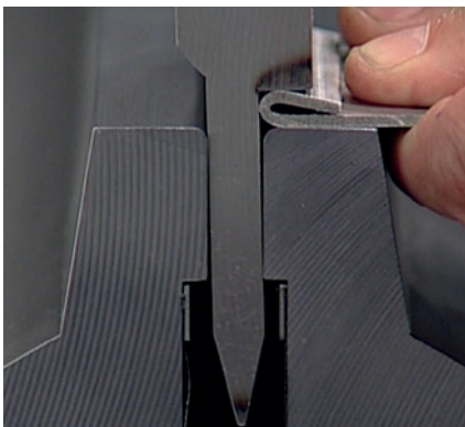
Pre-bend and flattening in the same tool.
